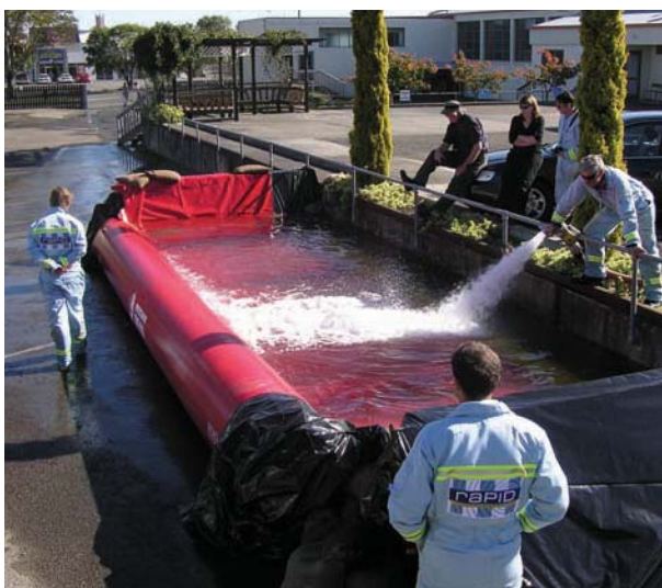
Flood barriers being tested as part of a RAPID flood training course.
